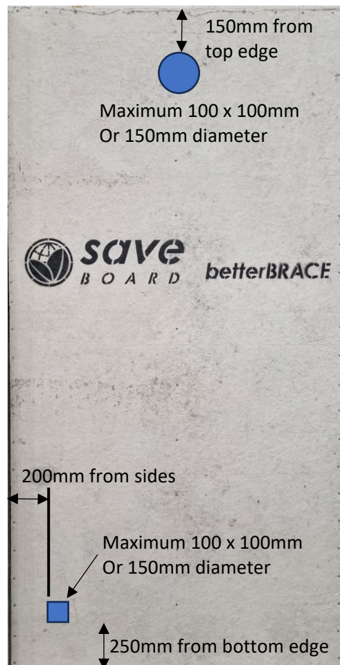
DIAGRAM 5 – Permitted penetrations in Bracing board. Note: All penetrations are to be sealed as per the instructions in this guide.
